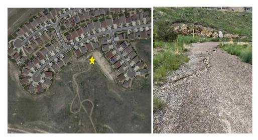
Keesen has identified multiple elements needing repair and restoration. The proposed plan is to start with correcting drainage points to ensure less future washout. Keesen has proposed an installation of catchment area on northside of path, where watershed is collecting, to reduce erosion of path and redirect majority of water. Proposed catchment will feed into drainpipe that will be trenched south, past bends of path and outlet, into native where riprap will be placed to dissipate flow.
